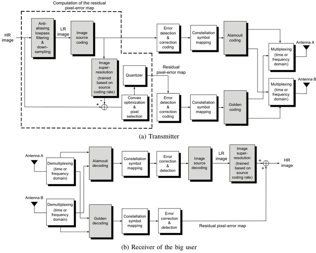
Fig. 1. The proposed MIMO image broadcasting system.
