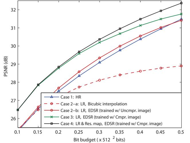
Fig. 2. PSNR performance of a big user in a SISO system with a bandwidth-limited, but error-free channel.
